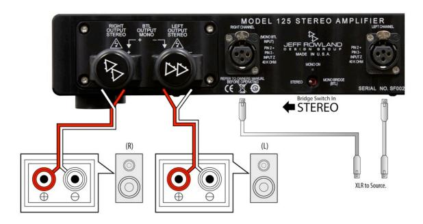
Figure 3: Stereo Mode loudspeaker connections
