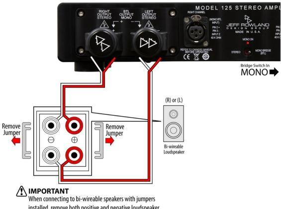
When connecting to bi-wireable speakers with jumpers installed, remove both positive and negative loudspeaker jumpers from binding posts. Failure to do so may result in damage to loudspeaker and/or amplifier.
