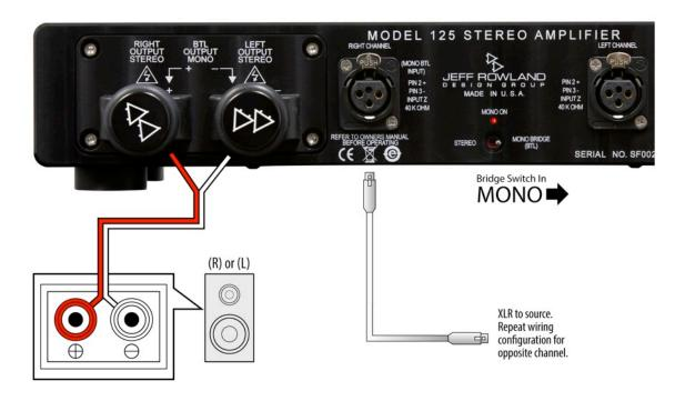
Figure 4: Bridge Mode loudspeaker connections
